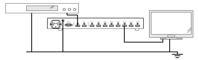
Fig. Connecting the FG terminals
